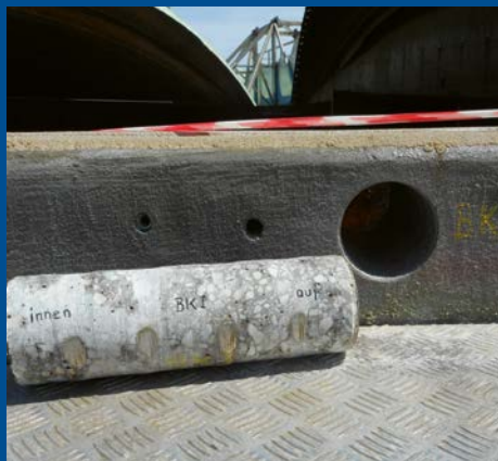
meaningful drilling cores for external laboratory testing
