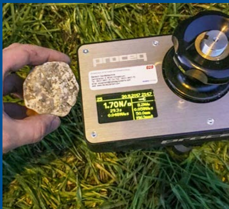
determination of adhesive tensile values
