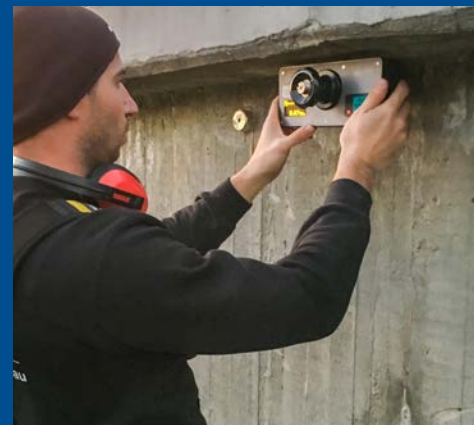
testing the tensile strength of the concrete
